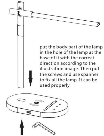
put the body part of the lamp in the hole of the lamp at the base of it with the correct direction according to the illustration image. Then put the screws and use spanner to fix all the lamp. It can be used properly.
